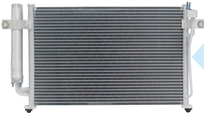
Hyundai Getz A07-7142 Multi-pass Condenser – not possible to successfully flush.
