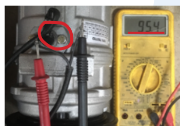
Fig. 2 Slip Sensor Ohmmeter reading 95.4 ohms
