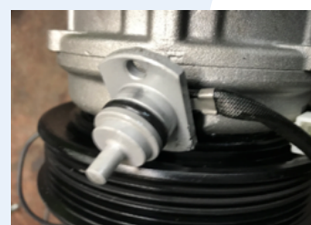
Fig. 3 Typical Slip Sensor pick up in Denso type Compressor
