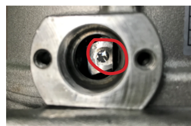
Fig. 4 View inside a compressor showing a magnet embedded in the crankshaft which creates a signal as it passes the slip sensor pick up unit in Fig. 3
